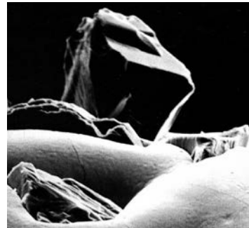
Diamond grinders: The surfaces of industrial diamonds are more regular. Therefore a somewhat coarser graining is selected (SEM image).
