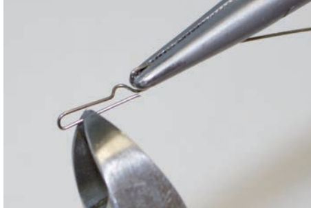
2. Shortening the bent brace ends
