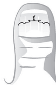
7 All wire parts that stick out are cut off as short as possible.
