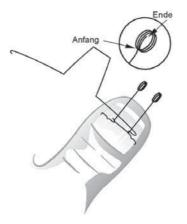
The loop is selected by visual judgement and wound round the small protrusions. The eye of the loop should be facing you. The loops are pressed together.
