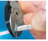
2. Cut off the Onyclip strip to the individual length required two different strengths are available
