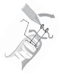
5. The winder is threaded through both eyes and positioned vertically.
